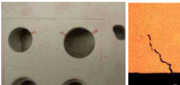
Figure 3: Hot tear located at a combustion chamber of a cylinder head
