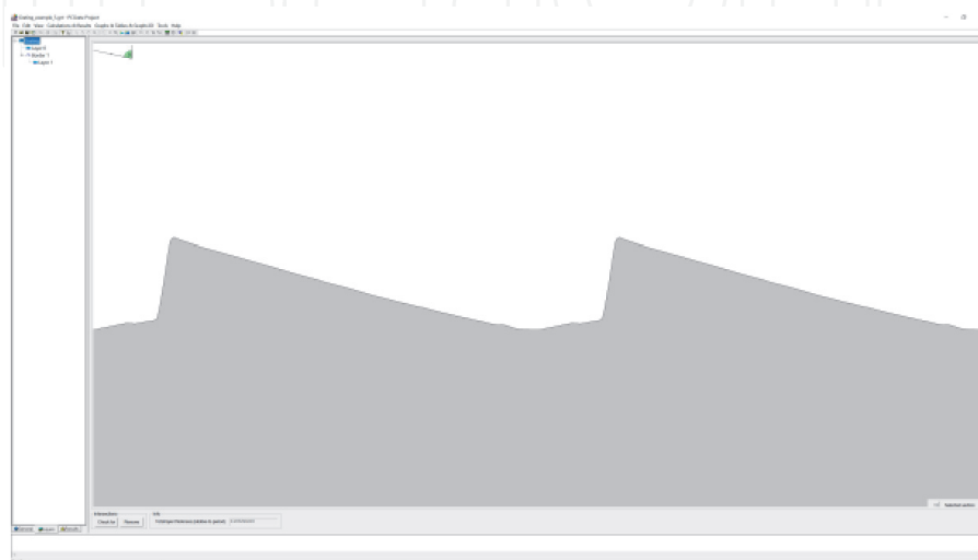
Figure 2. Average AFM groove profile for 112/mm echelle R5 grating.
