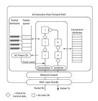
Fig. 3. Example of a communication data-path in a node.
