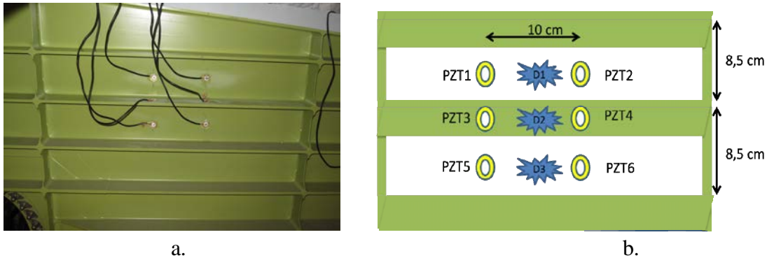
Figure 2. PZT's location and damage description.
