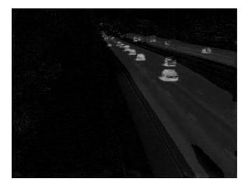
Fig. 7. Result of applying the probabilistic mask over the substracion of the background.
