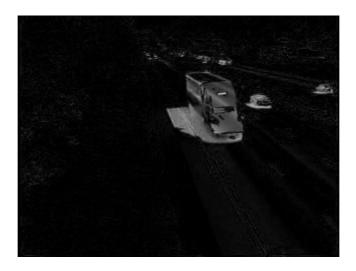
Fig. 3. Step 2, result of subtracting the background from the original image.
