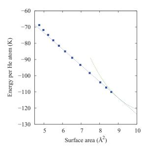
FIG. 2. (Color online) Energy per particle for a structure with a single layer triangular solid (dashed line) and a second layer liquid on top of a solid of density 0.115 Å<sup>-2</sup> (full squares) versus the inverse of the total helium density. The common tangent of a Maxwell construction is represented by a dotted line.
