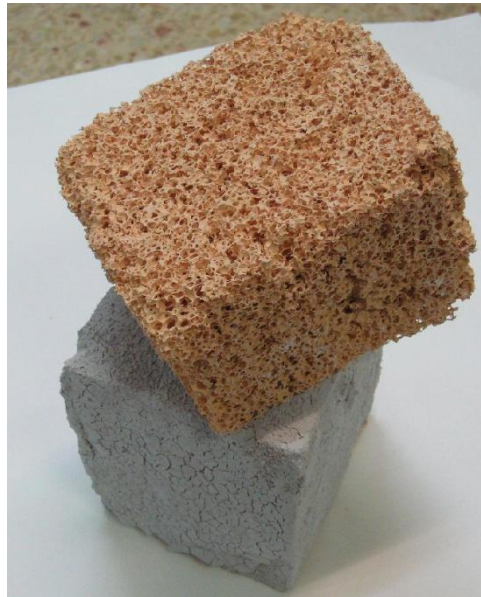
Figure 5. Thick-pore catalyst scaffold with and without outer coating, obtained in laboratory
