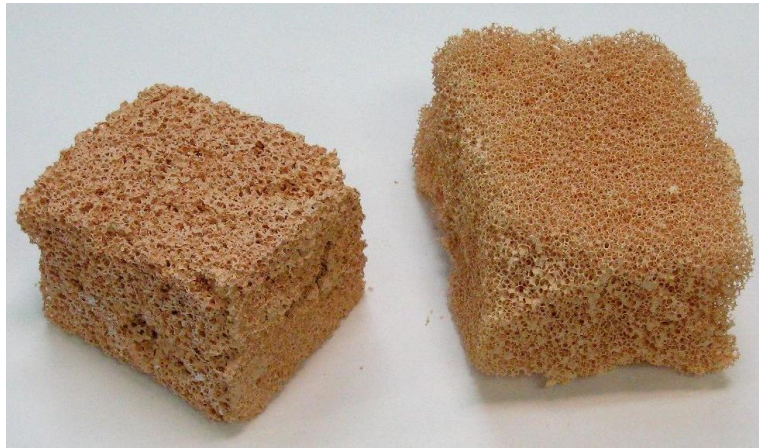
Figure 5. Thick-pore catalyst scaffold with and without outer coating, obtained in laboratory
