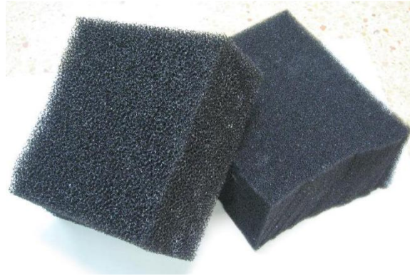
Figure 4. Catalyst scaffolds with thick and fine pores obtained in laboratory
