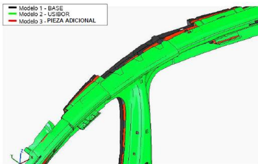
Figure 2: Comparison of plastic deformations in the upper A-pillar during Side Crash in the new Seat Ibiza. Comparative detail of plastic deformations in the upper A-pillar in side crash for the new SEAT Ibiza
