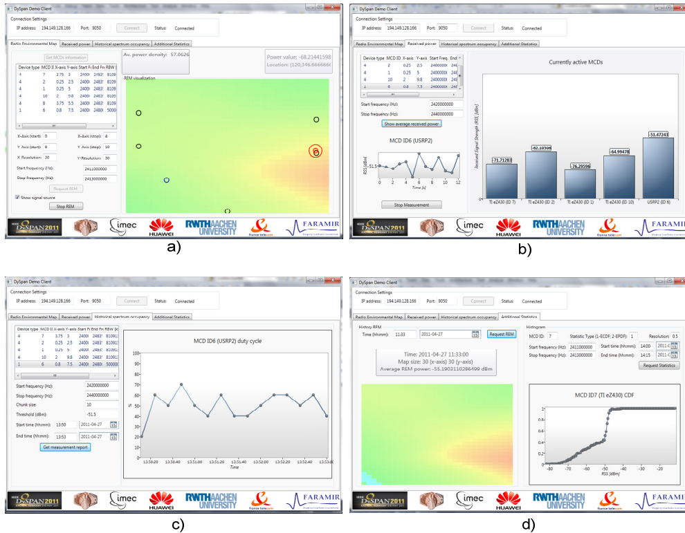
Figure 2-7: GUI's graphical data presentation a) REM screen with MCDs and estimated transmitter position b) Current RSS values for a single and multiple MCDs c) Calculated duty cycle for selected MCD d) Old REM and statistics graph
