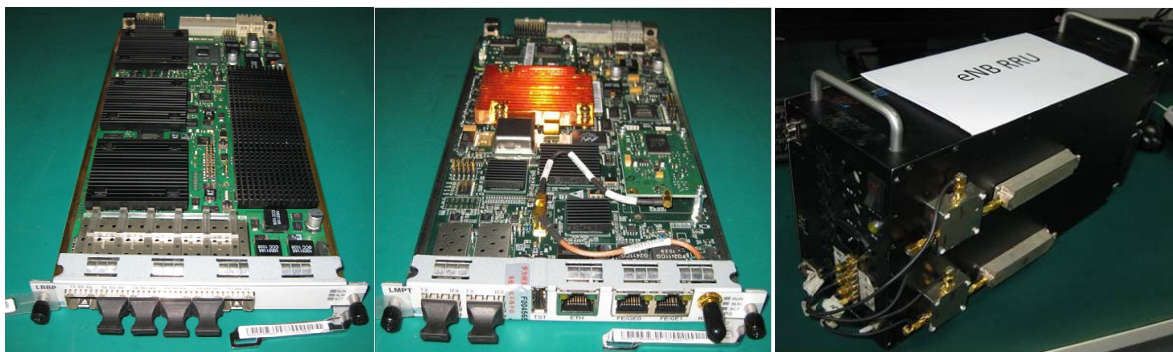
Figure 5-3: LTE eNodeB hardware - baseband board (left), transmission board (middle) and RF module (right).
