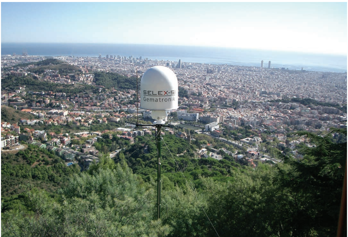
Visibility of the X-band radar located at the Fabra Observatory (414m AMSL) over the Barcelona metropolitan area
