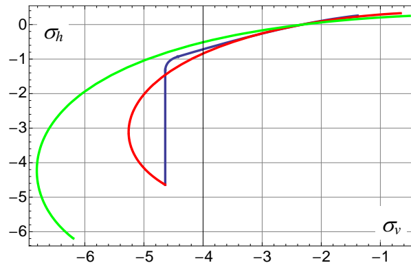
Figure 8: Leon (blue), Bresler-Pister 2D (red) and 3D (green) confined strength plots
