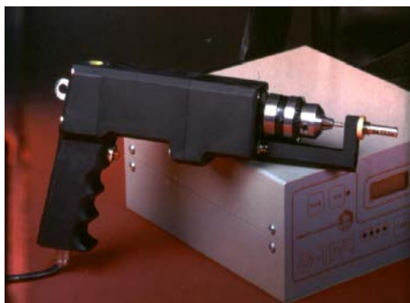
Figure 2: PNT-G penetrometer (a) and example of mortar strength measures (b)
