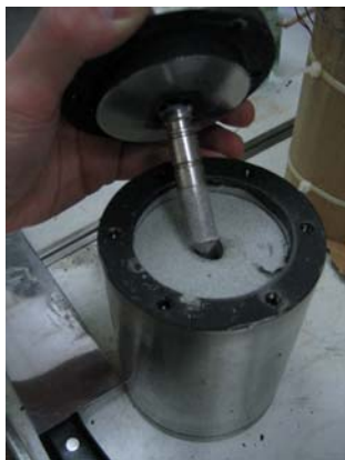
Fig.4 Appearance of the cell with the compacted bentonite inside, drilled to allow the entrance of the sensor.
