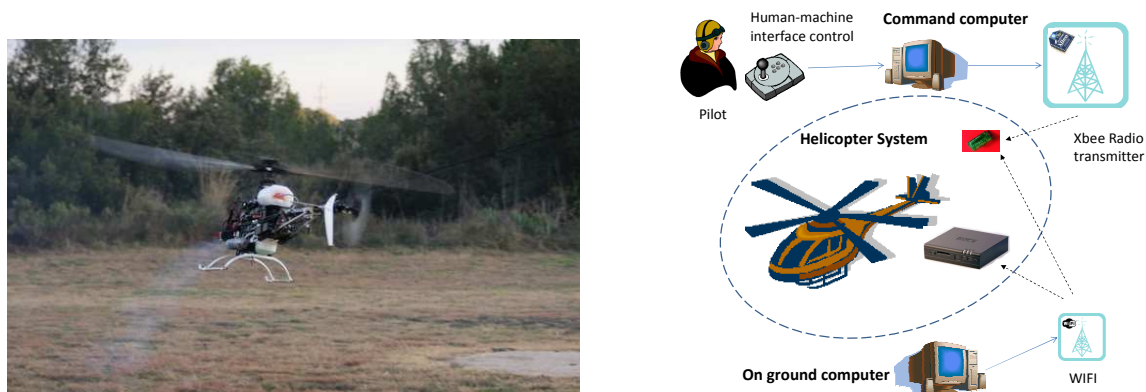
Figure 1: \alpha -SAC helicopter in autonomous flight (left) and block diagram (right)
