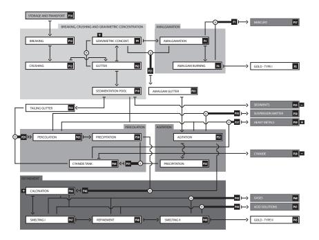
Figure 1: Example of flow diagram in a industrial process (premises).
