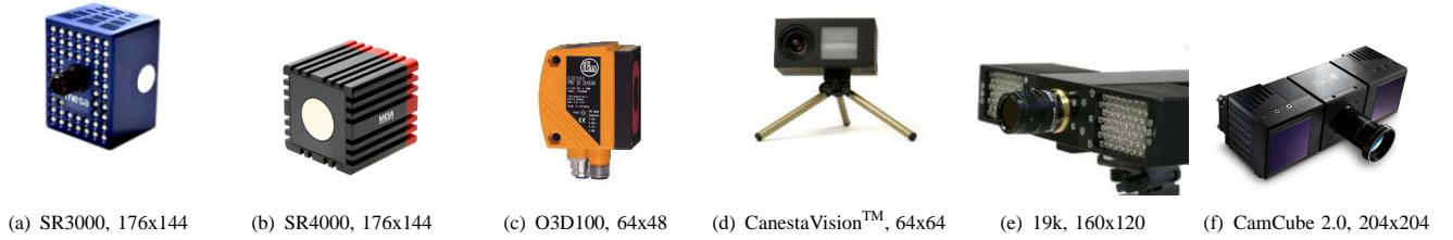
Fig. 2. Current commercial lock-in ToF cameras. (a-b) Mesa Imaging AG © [3]. (c) Ifm electronic © [4]. (d) CanestaVision ™ [5]. (e-f) PMD[Vision] ® [6]. Particularities of each solution include the use by CanestaVision ™ of square modulated waves [7], the use of a smart pixel - photonic mixer device (PMD) for simultaneous wave sensing and mixing by PMD[Vision] ® [8], and the addition by Mesa Imaging AG © of a coded binary sequence (CBS) modulation for multi-camera operation on SR4000 new models.
