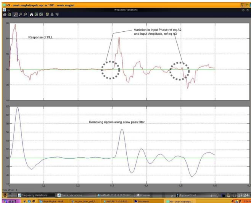
Figure B.3: Frequency Stabilization Using Comb Filter and Lagrangian, Length 1 Approximator by Varying Phase and Gain of s_1
