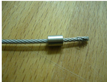
(a) Example of one side of the steel cable without the teflon cover and the end cap put in place.
