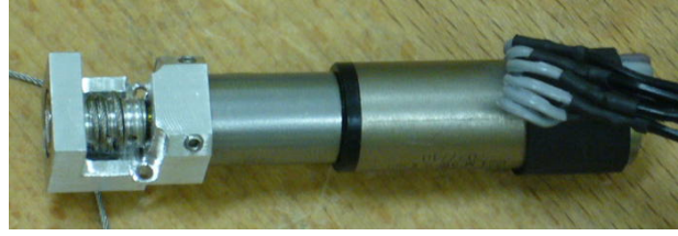
(a) Step 2 - Detail of the cable placed around the pulley of the proximal joints motors.
