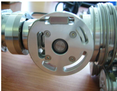
(a) First part that needs to be removed to assemble the cables 7 and 8.
