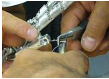
(a) Step 2 - Procedure to tighten the knot in the distal cables using two pliers.
