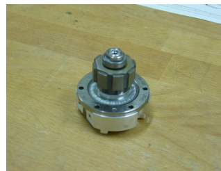
(b) Rotor of the motor which is attached to the harmonic gears to drive the cables.
