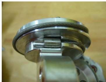
(a) Hole in the pulley with the shape of the end cap of the cable to attach it to the structure.
