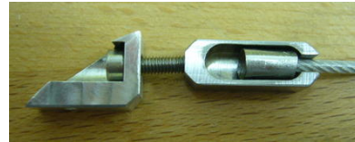
(b) Moving part where the other end of the cable is attached to adjust the tension of the cable.
