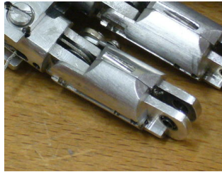
(b) Step 4 - Position of the proximal joint to make the first knot in the cable.
