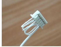
Figure 30: Connector used for the external fault input to split it in several independent wires to reach a set of motor control boards.
