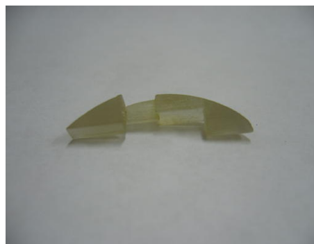
Figure 15: Plastic part used to fill the hole for the end caps of cables 1 and 3 to prevent cables 2 and 4 from getting into them.
