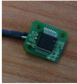
Figure 22: Detail of the board to acquire the position information from the Hall effect sensors.
