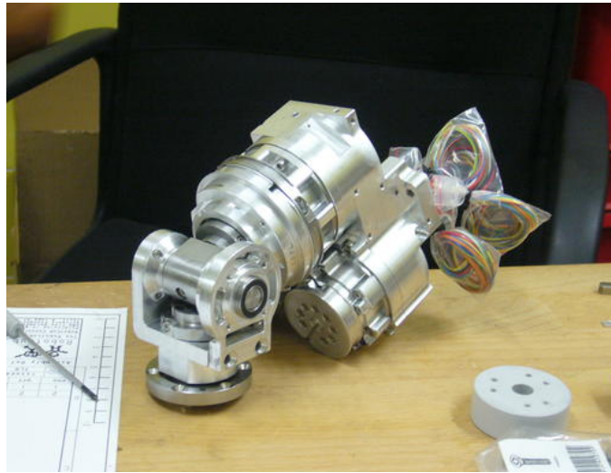
Figure 4: Picture of the shoulder of the icub robot fully assembled without the electronics.
