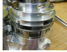
(b) Relative position of the two pulleys of the shoulder to place cables 2 and 3.
