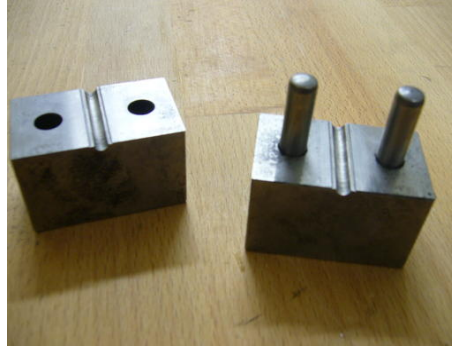
Figure 1: The two temperate steel parts used to crimp the end caps with the steel cables using the press. These two parts must be properly aligned using the marks in one of their sides (0).
