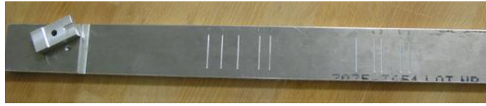
Figure 2: Ruler with marks for all the lengths of the steel cables used to avoid having to measure them each time.
