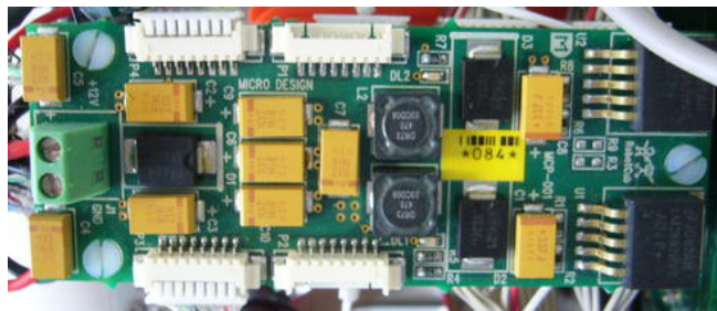
Figure 23: Detail of the board to provide the power supply up to 4 MC4 boards.
