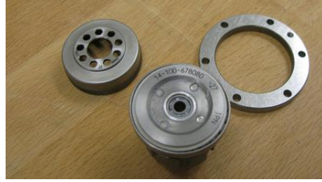
Figure 8: Detail of the three parts that make the harmonic gear used in the shoulder joints.
