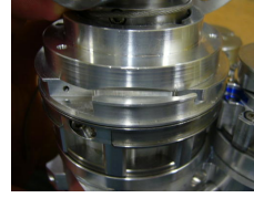
(c) Detail of the special shape of the third pulley from the left in Fig. 13(a) to insert cable 4.
