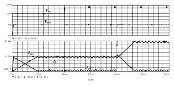
Fig. 5. Response of the converter shown in figure 2 with  $V_{in}$ =10 V. In addition, it can be seen the circuit response to a step of the input voltage from 10 V to 13 V at the time instant t=20  $\mu s$ , and a variation in the load resistance from 5  $\Omega$  to 2.5  $\Omega$  at t=40  $\mu s$ . The switching threshold current  $I_{\gamma}$  has been adjusted to 50 mA.
