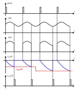
Fig. 7. Typical waveforms of one-cycle control.
