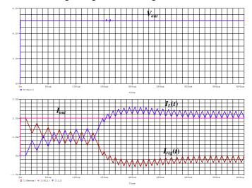
Fig. 10. Start-up transient waveforms when the current-mode one-cycle linear-assisted DC/DC converter provides 2 A at the output  $V_{out}$ . Notice that the one-cycle (20) control loop assures a value of the average current flowing through the linear stage
