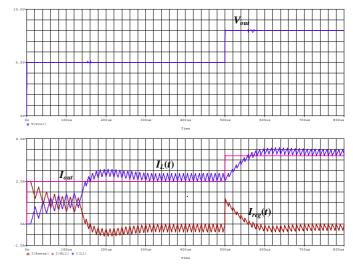
Fig. 11. Transient response of the linear-assisted DC/DC converter to a step when the reference voltage increases from 5 V to 8 V at 500  $\mu s$ .
