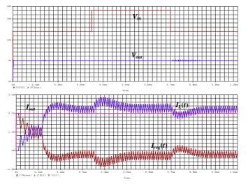
Fig. 13. Transient response when the input voltage has an increasing step from 12 V to 17 V (variation of 41.7%) at  $t=350 \mu s$  and vice versa at  $t=700 \mu s$ .
