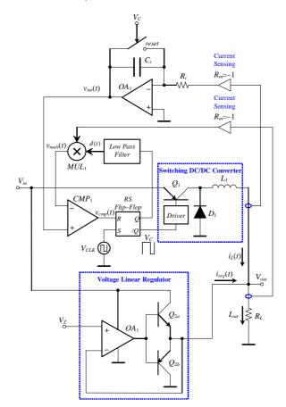
**Fig. 8.-** Basic structure of a current-mode one-cycle linear-assisted DC/DC converter.
