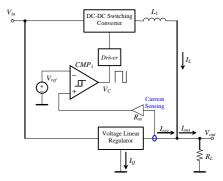
Fig. 1. Block diagram of the proposed linear-assisted converter.
