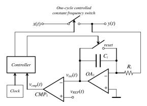
Fig. 6. Basic scheme of one-cycle control.
