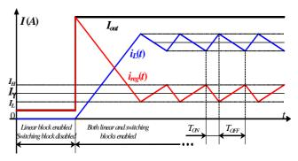
Fig. 3. Principle of operation of the proposed linear-assisted DC/DC converter.
