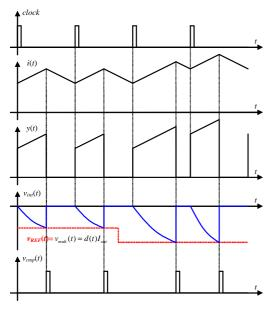
Fig. 9. Typical waveforms of the proposed linear-assisted converter with current-mode one-cycle control.
