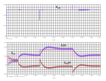
Fig. 12. Transient response when the output current has an increasing step from 2 A to 3.33 A (variation of 66.6%) at t=350  $\mu s$  and vice versa at t=700  $\mu s$ .
