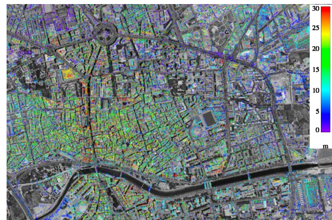
Figure 5 Retrieved height error in the city. Higher errors are located along the main streets of the city where taller buildings are located.
