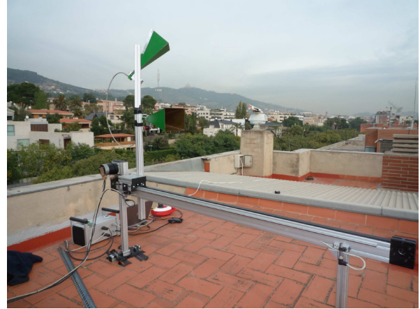
Fig. 3. Controlled moving target consisting on a BARC attached to a linear unit.
