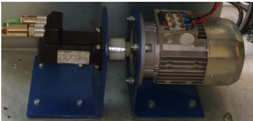
Comparison between a PMSM and an IM with the same power
