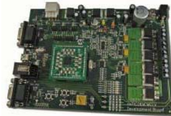
Electronic board to control a BLDC motor
