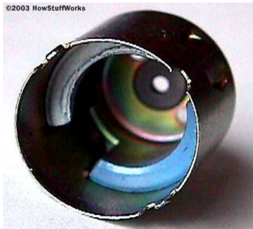
2 and 6-poles permanent magnet stators (fields)
