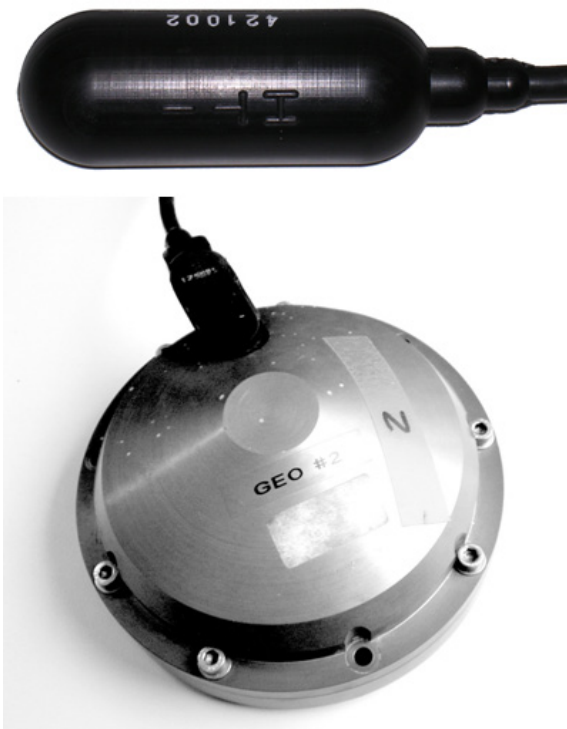
Figure 1: Hydrophone (on top) and geophone (on bottom)
