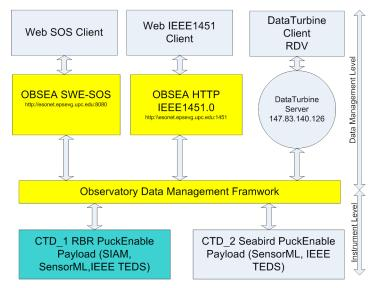
(before) Figure 2 Access to real-time data using standards like SWE SOS or IEEE1451
