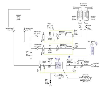
Fig. 1 Diagram of the pneumatic and hydraulic systems
