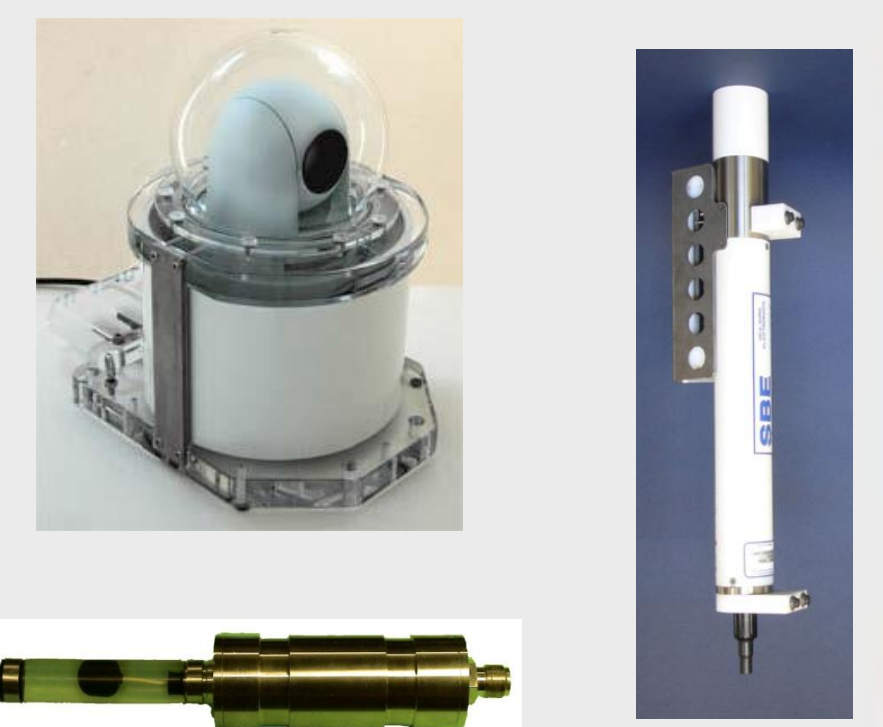
SeaBird CTD Instrument Biore Naxys Ethernet hydrophone Ocean Presence underwater IP camera system
