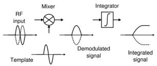
Figure 3. Impulse radio correlator operation.
