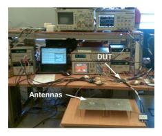
Figure 7. Measurements testbench setup.
