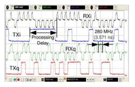
Figure 8. Datagram measurements of the transmitted bits and the demodulated signals at 560 Mbps.
