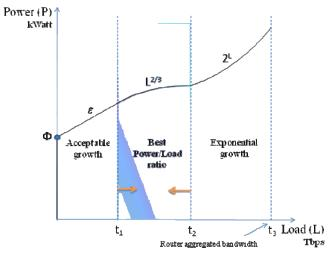
Figure 3. Power consumption in combined power consumption model.
