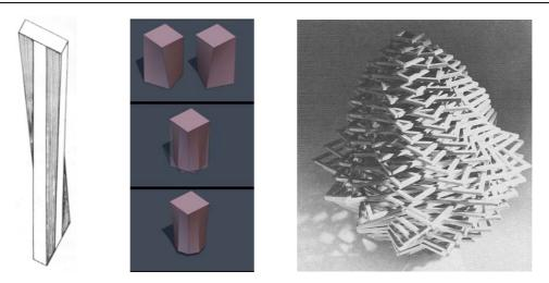
45.-The varying character of things is not taken into account in the most of the cases. This column made with transitional surfaces and rectangles is rarely times described in terms of its varying section. *Savona Railway Station* by Antonio Nervi and Pier Luigi Nervi.
