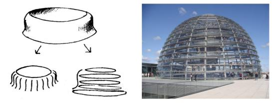
1.-There are two possible interpretations of this pattern, the first is the revolution of a curve around a circle and the second is a description where the horizontal section of the object is variable. Because of its regularity the first option is the simplest and the one we use as a description of the object. [20]
