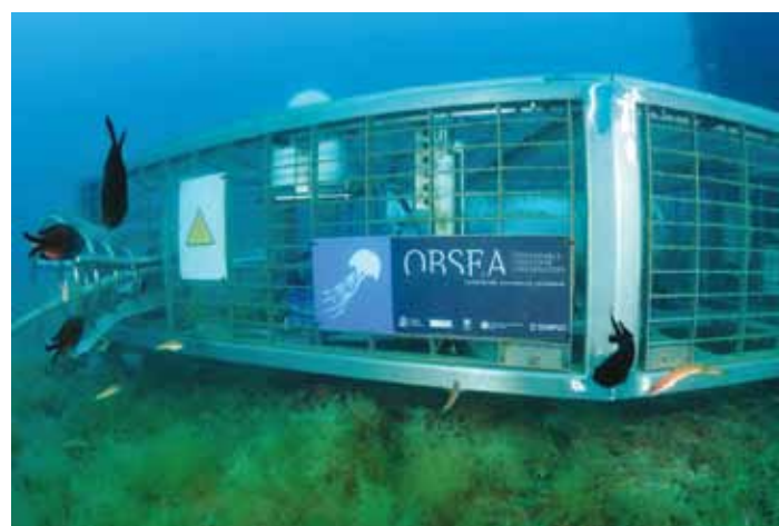
Fig.3 - OBSEA Structure: this cabled observatory is located in 10 m depth and is now operational for one year.
