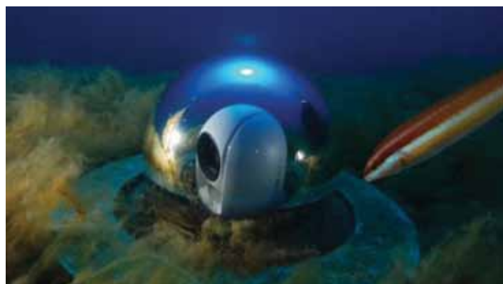
Fig.8 - Underwater camera at OBSEA observatory. The system is remotely controlled via a standard communication link
