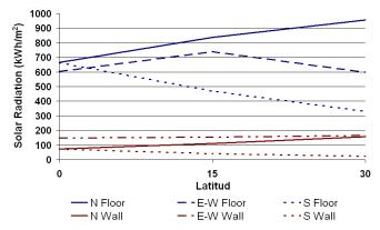
Fig. 11 Effect of latitude on total incident solar radiation in a year
