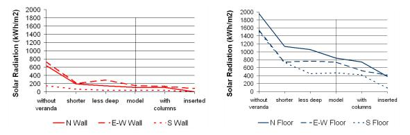
Fig. 12 Overall comparison of total annual incidence of solar radiation at 15°S.
