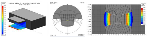
Fig. 8 Solar radiation on floor Fig. 9 Masking graph and wall from Dec. to Jan.
