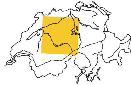
Fig. 4. Domain ( 100 \cdot 100 \text{ km}^2 ) of radar composites used in present analysis. The grid spacing is 1 km.
