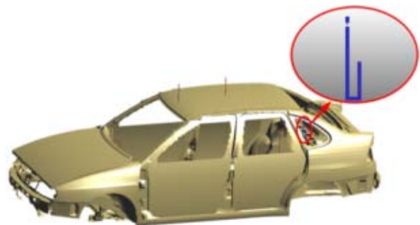
Fig 9. M3a and M3b antenna details in the car model.
