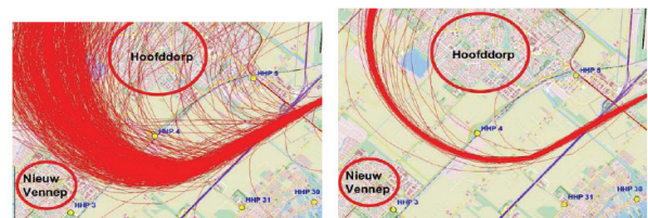
Figure II-3: Example of flight tracks corresponding to the initial turn of the Spijkerboor departure in Schiphol (The Netherlands)
