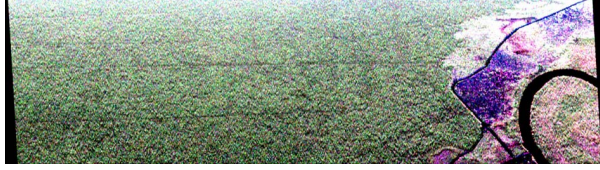
Fig. 4: Pauli RGB decomposition of the Master data set ( R = |S_{hh} - S_{vv}| , G = \sqrt{2}|S_{hv}| , B = |S_{hh} + S_{vv}| )
