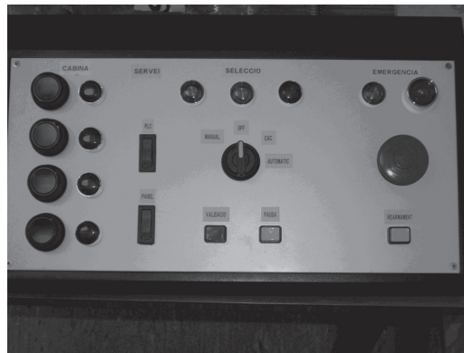
Figure 3: The human operator can intervene inside the automation cycle (GRAF CET transition) with the use of an industrial panel. In this panel the human operator follow the functional operational modes of the GEMMA guide.
