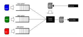
Figure 3. ONU functional schema
