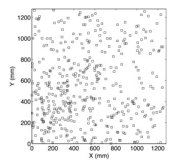
**Fig. 4.** Digitized version of Fig. 1a of Schertzer and Lovejoy (1989) (equivalent to Fig. 1 of LS) with the approximate locations of 438 of the original 452 raindrop stain centers collected on a  $128 \times 128 \, \mathrm{cm}^2$  chemically treated blotting paper during an exposure time of approximately 1 s.
