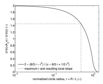
**Fig. 3.** The local slope of the bold line in the bottom panel of Fig. 2 as a function of the normalized circle radius r=R/L (bold line). The dashed line indicates the maximum normalized circle radius considered by LS and the corresponding local slope. Note that the validity of our analytical solution (Eq. 2) is limited to the interval  $0 \le r \le 1$  (the solution for the remaining interval  $1 \le r \le \sqrt{2}$  is presented elsewhere).
