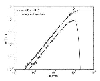
**Fig. 7.** The same analysis as Fig. 5, but applied to the spatial point pattern of Fig. 6. Note that the fractal correlation dimension determined for this homogeneous realization (1.92) is the same as that for the supposedly fractal point pattern of Fig. 4.
