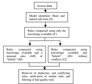
Figure 2. Ordered steps of the rule extraction method.
