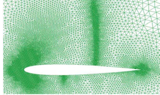
Figure 2 b: Final (right) mesh around NACA 0012.
