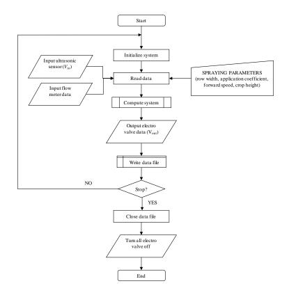
Figure 2.Flow chart of the whole electronic system for variable application
