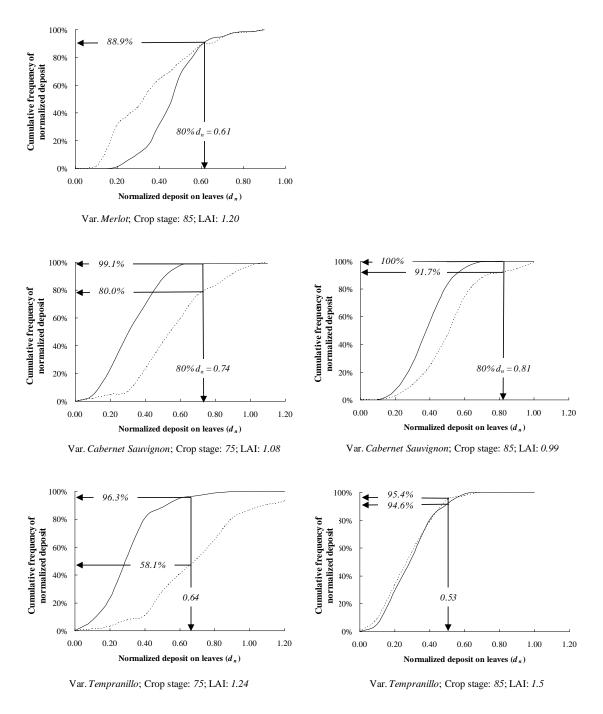
Figure 3. Cumulative frequency of normalized deposit on total leaf samples and cumulative number of samples below 80% of theoretical normalized deposit. Results for conventional application (-----) and proportional according sensors measurements (-----)
