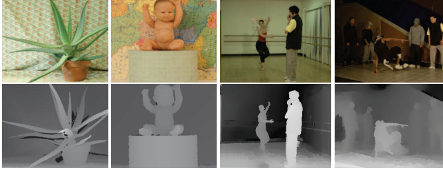
Fig. 2: From left to right: Aloe and Baby1 datasets (from [8]), Ballet and Breakdancers (from [9]); including one of the color views (top) and its corresponding disparity map (bottom).
