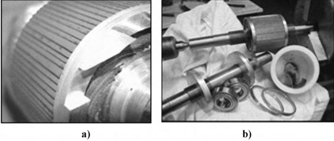
Fig. 6. Rotor with spiral sheet in manufacturing phase. a) Type A, b) Type Z.
