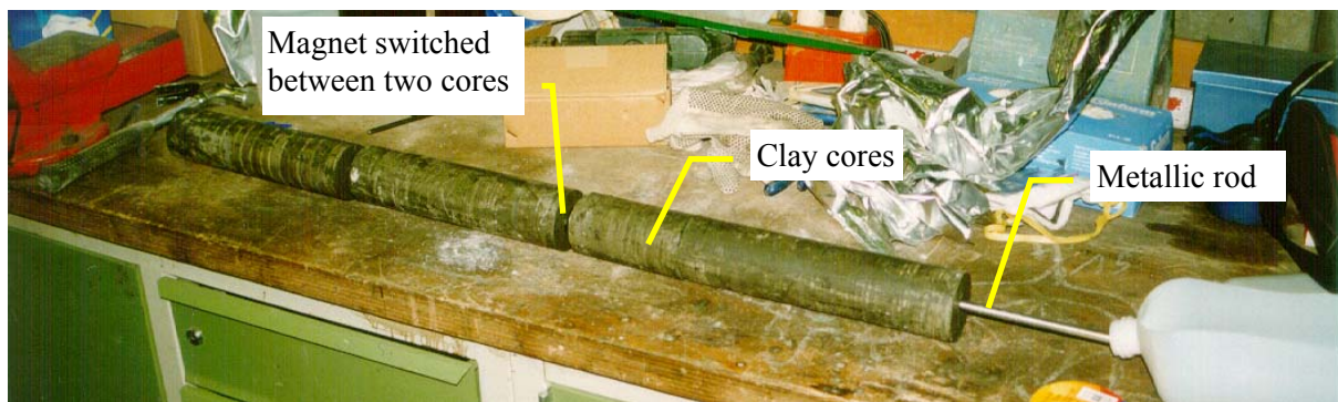
Figure 4-15: Picture of the installation of the displacement sensors. The metallic rod is inserted into the centre of the clay cores and two magnets are sandwiched between the clay cores.
