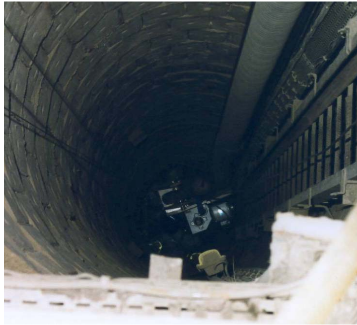
Figure 4-8: Top view of the vibro-compactor designed for the shaft sealing test (left) and a picture of the compactor in the shaft (right).
