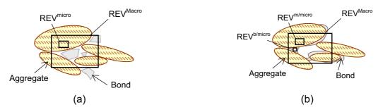
Figure 2. Conceptual representation of a bonded expansive material. (a) for Model 1 and (b) for Model 2.
