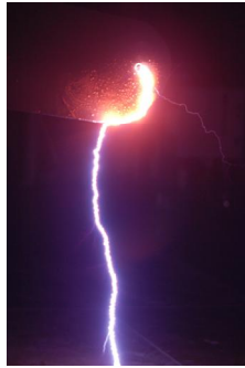
Figure 5. Picture of the breakdown when the blade is full polluted with salt mist.
