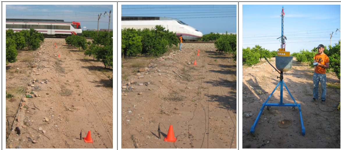
Figure 5. Two types of the measured trains at the test site and a view of the drop-weight used to characterize the ground.
