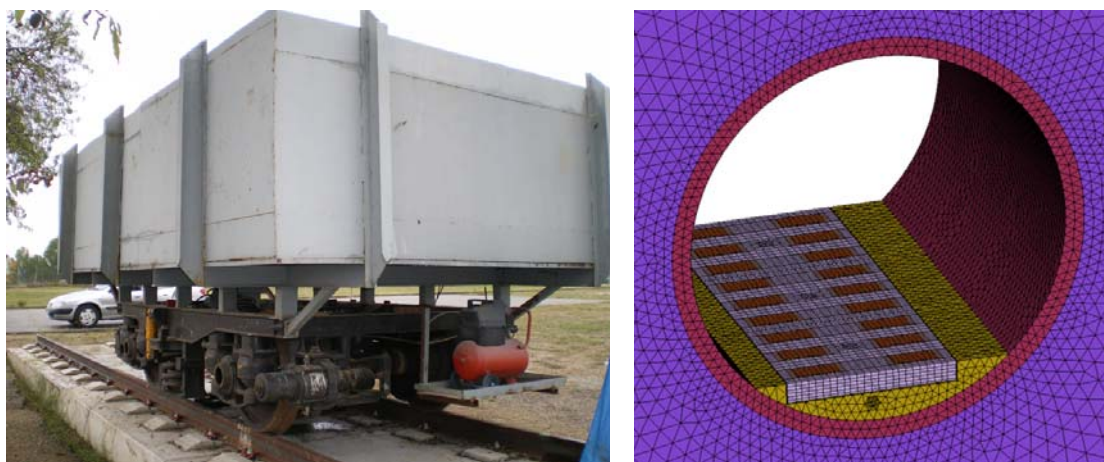
Figure 6: Test rig (left hand) and floating slab system FEM model (right hand)
