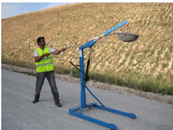
Figure 5 – Impactor developed by SENER (left hand) and ground vibration propagation results from SASW (right hand)
