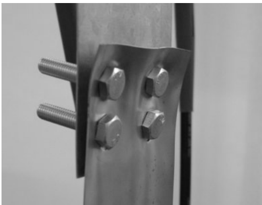
Fig. 5. Tilting + bearing in specimen 0,85-1-10-2-S250.
