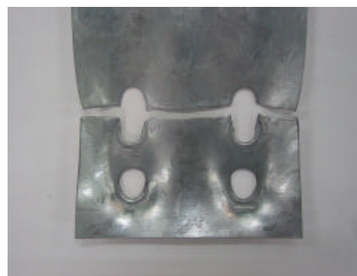
Fig. 6. Net section failure in specimen 1-1.5-10-2-S250.
