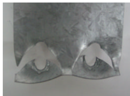
Fig. 8. Bearing failure in specimen 1-1-10-1-S250-A.
