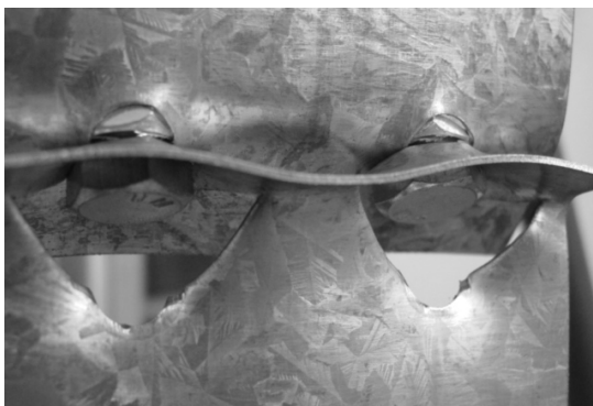
Fig. 21. T+B+TS failure of specimen 1-1-10-1-S250-A, without washers.
