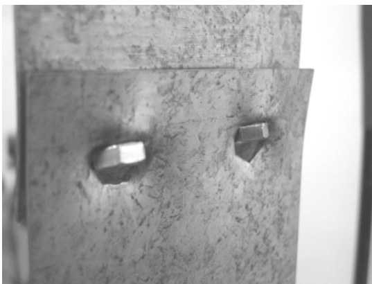
Fig. 31. Failure of specimen 1,5-1,5-8-1-S250.
