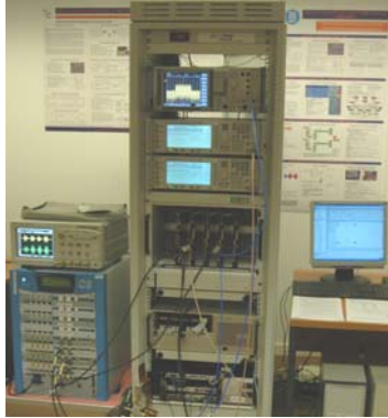
Figure 8: CTTC real-time testbed. Left: channel emulator, oscilloscope. Rack: (top to bottom) spectrum analyzer, signal generators, RF frontends, baseband boards.
