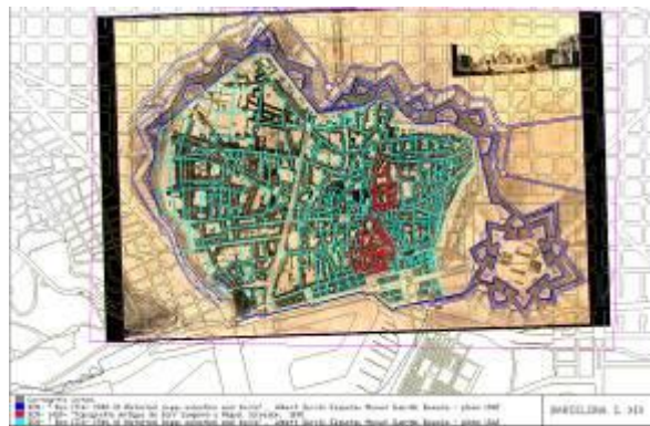
Figure 1. Superposition of a 19th Century City Plan adjusted and Modified to meet the precision of today's cartographic plans
