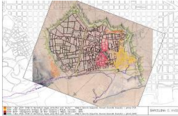
Figure 3. Superposition of an 18th century City Plan adjusted and modified to meet the precision of today's cartographic plans.
